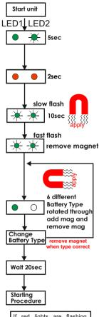
If red lights are flashing alternatively then you have to reconnect your yellow/black to 12V to reinstate the remote control. To set unit back to automatic mode swipe the magnet across the swipe area.
