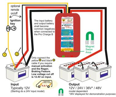
Battery Chemistry Profiles - magnet (enclosed) required to swipe, on start up, to change battery type. LED sequence cycles through as below.
